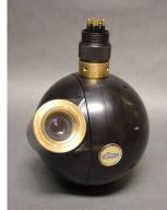
Variable speed pan and tilt, automatic or manual focus and two speed power zoom are all controlled remotely from one of a range of control units.
