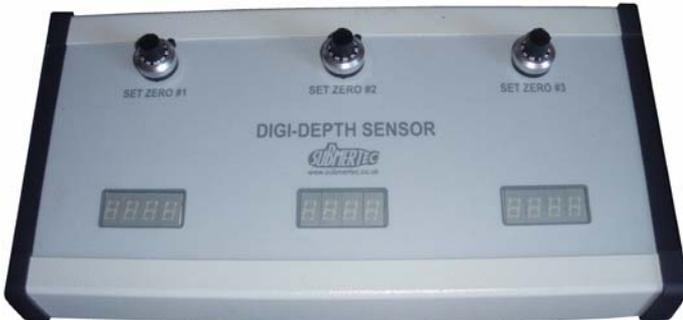
An easy to use and rugged digital depth measuring system consisting of high accuracy pressure probes, underwater cables and a desktop display unit with triple digital displays.
